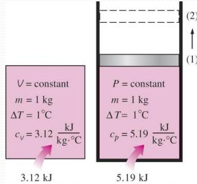
Constant volume, for which the work term (P dV) is zero, so that the specific heat (at constant volume) is
