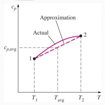
For small temperature intervals, the specific heats may be assumed to vary linearly with temperature.
