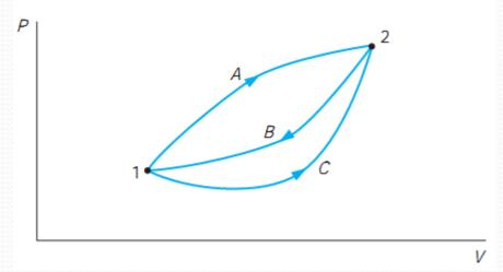
Since A and C represent arbitrary processes between states 1 and 2, the quantity  $\delta Q - \delta W$  is the same for all processes between states 1 and 2. Therefore,  $\delta Q - \delta W$  depends only on the initial and final states and not on the path followed between the two states. We conclude that this is a point function, and therefore it is the differential of a property of the mass.
