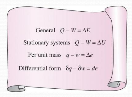
Various forms of the first-law relation for closed systems when sign convention is used.(For a stationary system  $\Delta KE = \Delta PE = 0$ ) The first law of thermodynamics for a change of state may therefore be written
