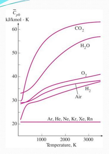
Some observations can be made from Figure. First, the specific heats of gases with complex molecules (molecules with two or more atoms) are higher and increase with temperature.
